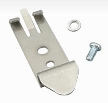
The DIN rail clip is made of zinc plated steel, used to mount items to 35mm DIN rail, 4mm mounting hole size.
